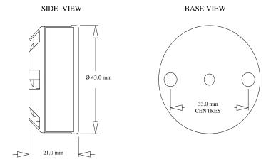
Fixing holes 2 x  $\emptyset$ 5.5 mm, Centre hole  $\emptyset$ 4.5 mm
